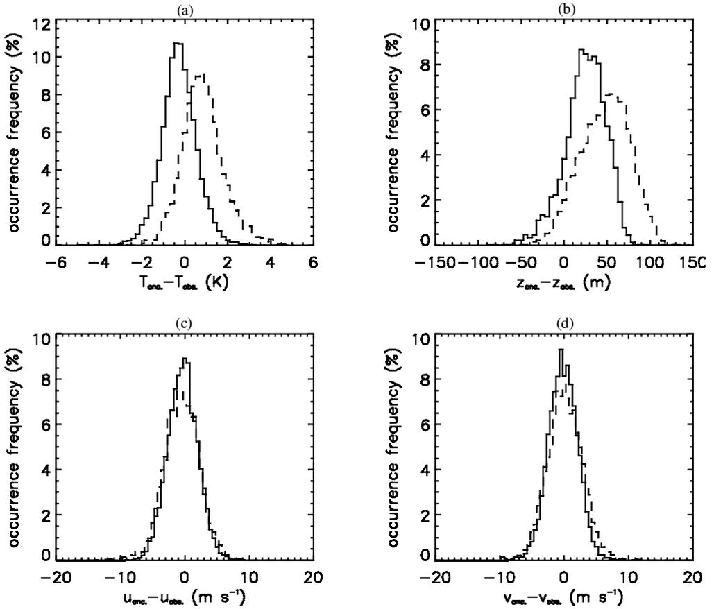
Figure 4. Histograms of differences—analyses (ECMWF solid, NCEP dashed) minus balloon observations: (a) temperature, (b) altitude, (c) zonal speed and (d) meridional speed.
