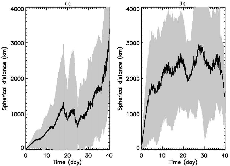
Figure 8. Mean (solid line) and standard deviation ( $\pm 1\sigma$ ) (grey shading) of separation distance between real and simulated SPB trajectories as a function of the elapsed time since the simulated SPB launch. Simulations were computed with (a) ECMWF and (b) NCEP winds.
