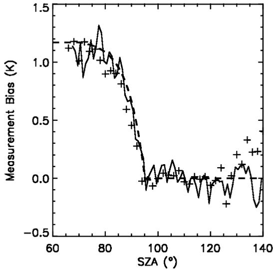
Figure A.1. Determination of the daytime bias in temperature measurements; empirical result from observations (solid line), the modelled correction scheme (heavy dashed) and ECMWF–observation differences when the heating correction is not applied (crosses).
