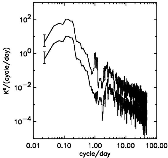
Figure A.2. Frequency spectra of temperature fluctuations during the SPB6 flight, computed from raw temperature measurements and after the heating corrections have been applied. For clarity, this latter spectrum has been shifted downwards by one decade. The error bars show the 90% confidence levels.
